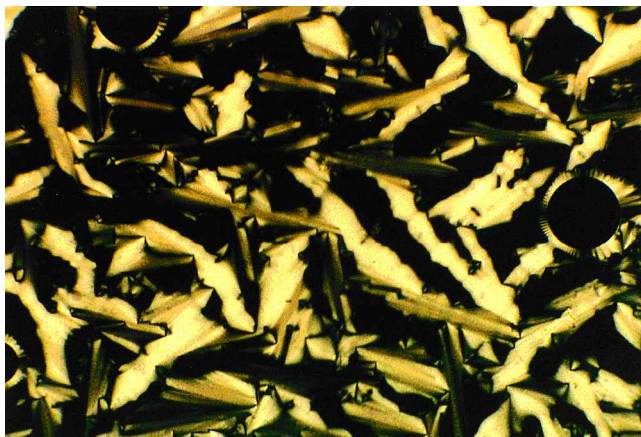
Figure 5. Optical micrograph ( \times 200 total magnification) between crossed polarizer of MTAI containing 20 wt % of dimethyl sulphoxide on being cooled from the isotropic phase to 329 K.
